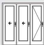
Pattern 330 2 Fold&Slide sashes 1 Turn-Only sash
